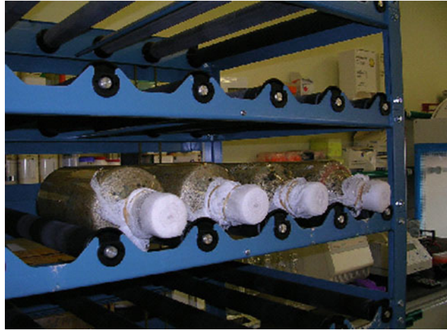
Fig. 2. The FERMEX method. Roller bottles (2 l) on roller bottle machine. Note cellulose closures fastened in place with gauze and rubber bands.
