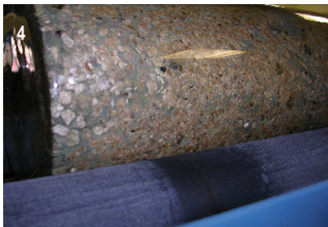
Fig. 4. The FERMEX method. Mycelium and vermiculite matrix formed by Trichoderma virens on roller bottle wall.
